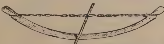
Fig. 54.—Spanish Windlass (for bending wood)
